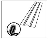
3. Using heavy snips, notch standing seam at bend points.
