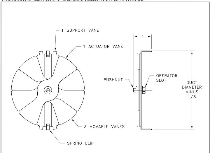
Model R-42 dampers feature gang operated radial blades that move in right angles to the air flow to regulate air volume. A flat configuration with no adapter ring enables the damper to be mounted flush with the neck of diffuser. Adjustments are easily made from the face of the diffuser with a screwdriver. Available in 6", 8", 10", 12" and 14". Steel construction. Mill Finish.
